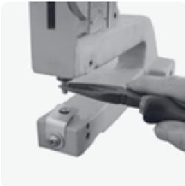
6. Now carefully pull the pilot pin out of the cylinder with pliers.
