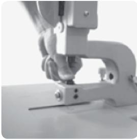
9. Insert the lower punch from the conversion kit and set it as far down as possible with the adjusting screw.
