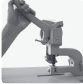
14. Now adjust the lower punch with the adjusting screw such that there is the correct distance for the material to be eyed and lock it in this position with the fastening screw.
