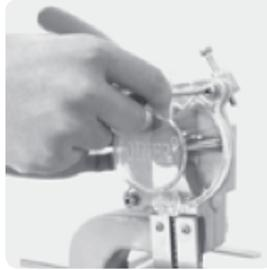
2. Loosen both fastening screws on the magazine cover and remove the magazine cover.
