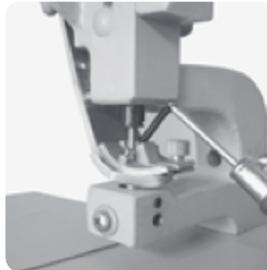
4. Now loosen the fastening of the return spring and remove the eye channel.
