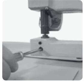
15. Finally, insert the wiping spring, align it with the lower punch and secure it.
